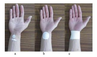
Figure 1. Pressure sensor is set on the palmaris longus muscle tendon
