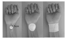
Figure 4. (a) only sensor, (b) sensor with cover tape, and (c) wrist taping with sensor and wrapped cover tape
